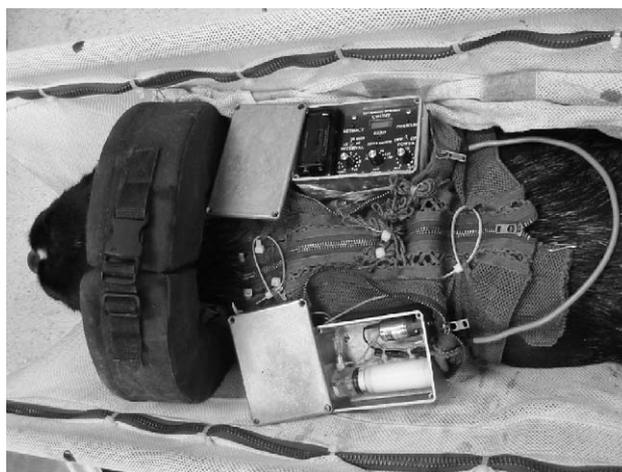
Fig. 4. Photograph depicting the aluminum boxes containing the electrical and mechanical components of the automated hydraulic coronary occlusion device stored in the jacket pockets of a typical conscious, chronically instrumented dog.
