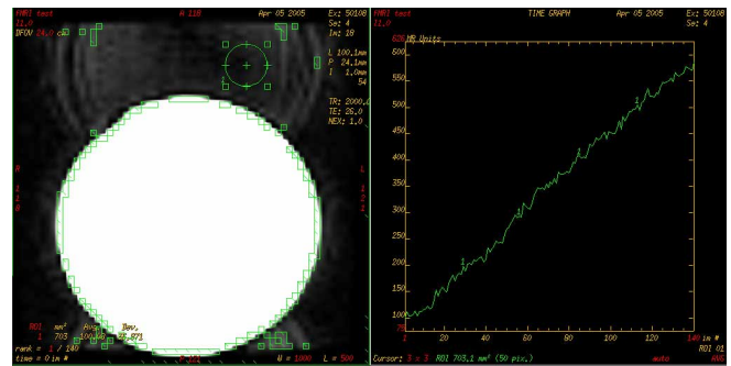
Fig. 1. Single-channel 3T fMRI ghosting levels without dynamic EPI phase correction.
