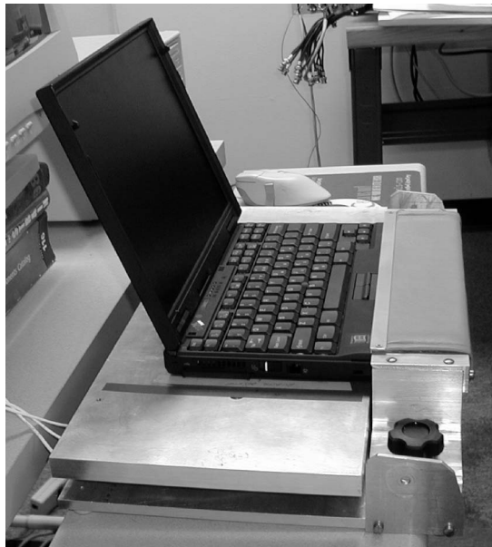
Figure 5. Keyboard force fixture with notebook computer and wrist support.
