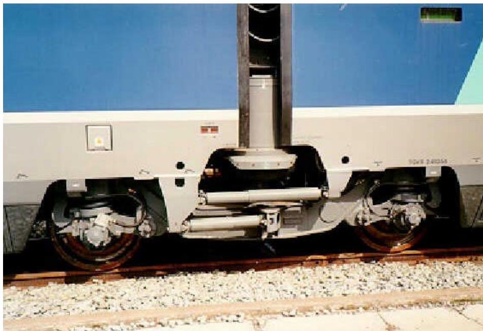
**Figure 1** Articulated joint and shared truck concept of the French TGV<sup>1</sup>.
