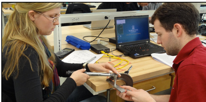
Figure 21: Measuring bolt clamping force in Experiment 7.
