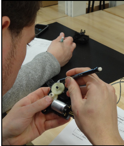
Figure 13: Counting gear teeth in HVAC baffle drive in Experiment 4.
