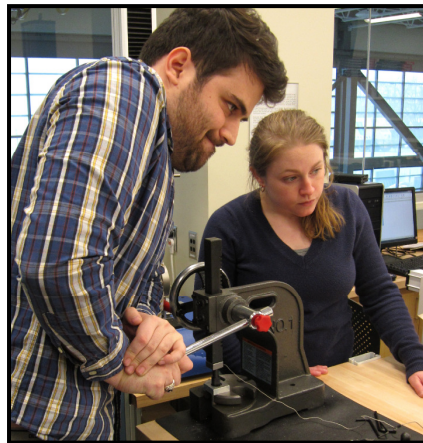
Figure 11: Press fit using an arbor press in Experiment 3.
