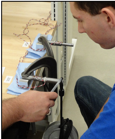
Figure 8: Measuring strain in round stock with stress concentrations in Experiment 2.
