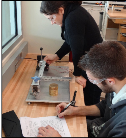
Figure 7: Measuring bending and torsional strain in Experiment 2.
