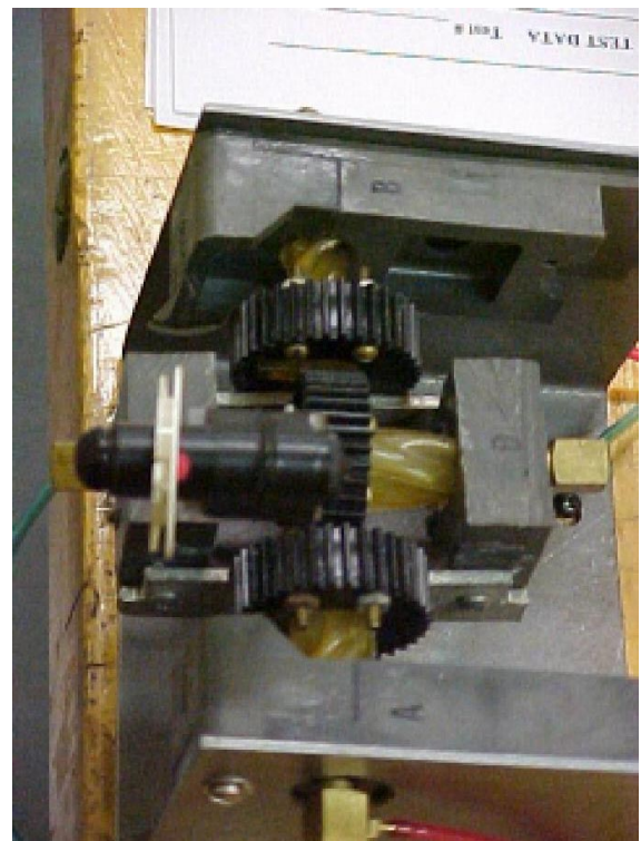
Fig. 6, Two Opposed Twistor-Pairs in an orthogonal configuration forming a Gimbal-drive
