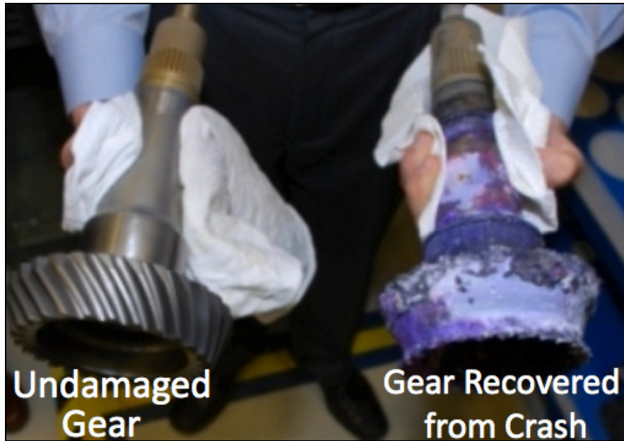
Figure 9. Failed Gear Comparison http://www.flightglobal.com/blogs/as-the-croft-flies/2009/06/feds_sikorsky_too_little_too_late_on_cougar_s-92_crash/
