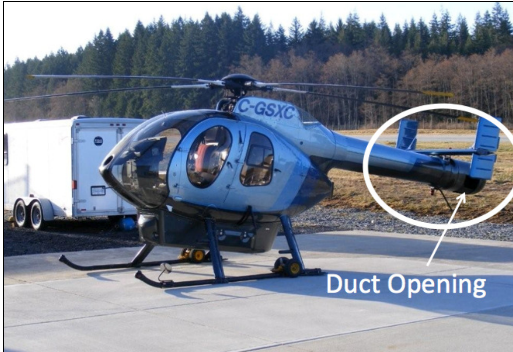
Figure 7. Shaftless Anti-torque System http://jetav.com/md-520n-specifications/
