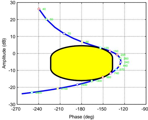
Fig. 2. Nichols plot for  $M = 1.46$  and  $K = 2$ , corresponding to  $40^\circ$  phase margin or greater and 16 dB gain margin or greater. The open-loop must not enter the shaded region in order to satisfy the  $M, K$  constraint.
