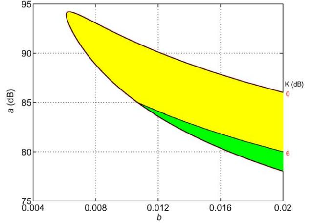
Fig. 1. Region of  $(a, b)$  values for  $M = 1.46$ , equivalent to  $40^\circ$  phase margin or greater and 10 dB gain margin or greater. Lower shaded region is with additional 6 dB plant gain uncertainty ( $K=2$ ) for a total of 16 dB or greater.
