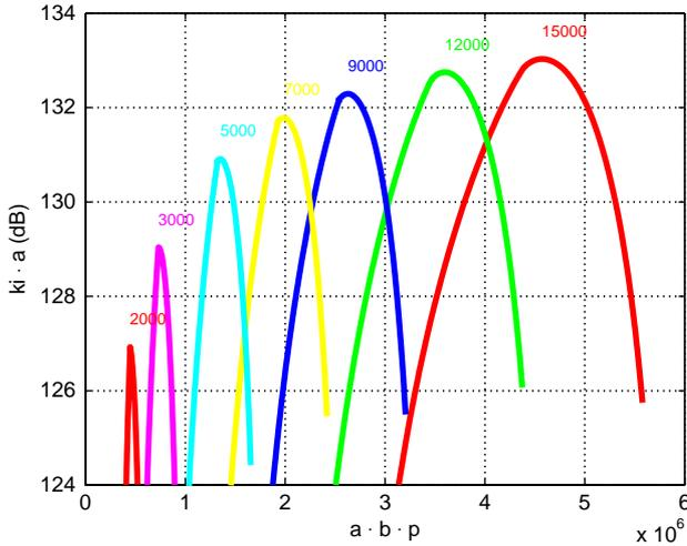
Fig. 3. Region of  $(ak_i, abp)$  values for  $M = 1.46$  and  $K = 1$ .
