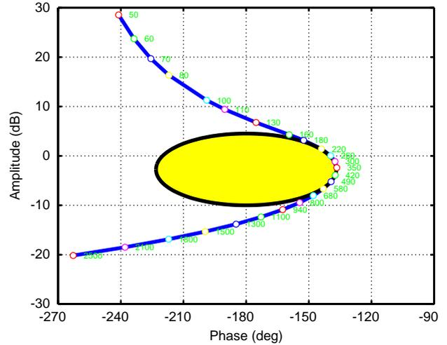
Fig. 4. Nichols plot for  $M = 1.46$  and  $K = 1$ . Frequencies are marked in rad/s. The open-loop transfer function must not enter the shaded region in order to satisfy the  $M$  and  $K$  constraint.
