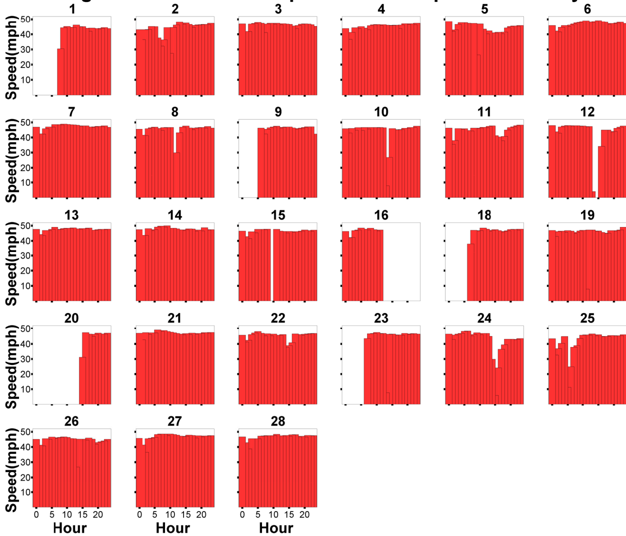
A4 Figure 15. Control Ramp: Detector D Speeds February 1999.
