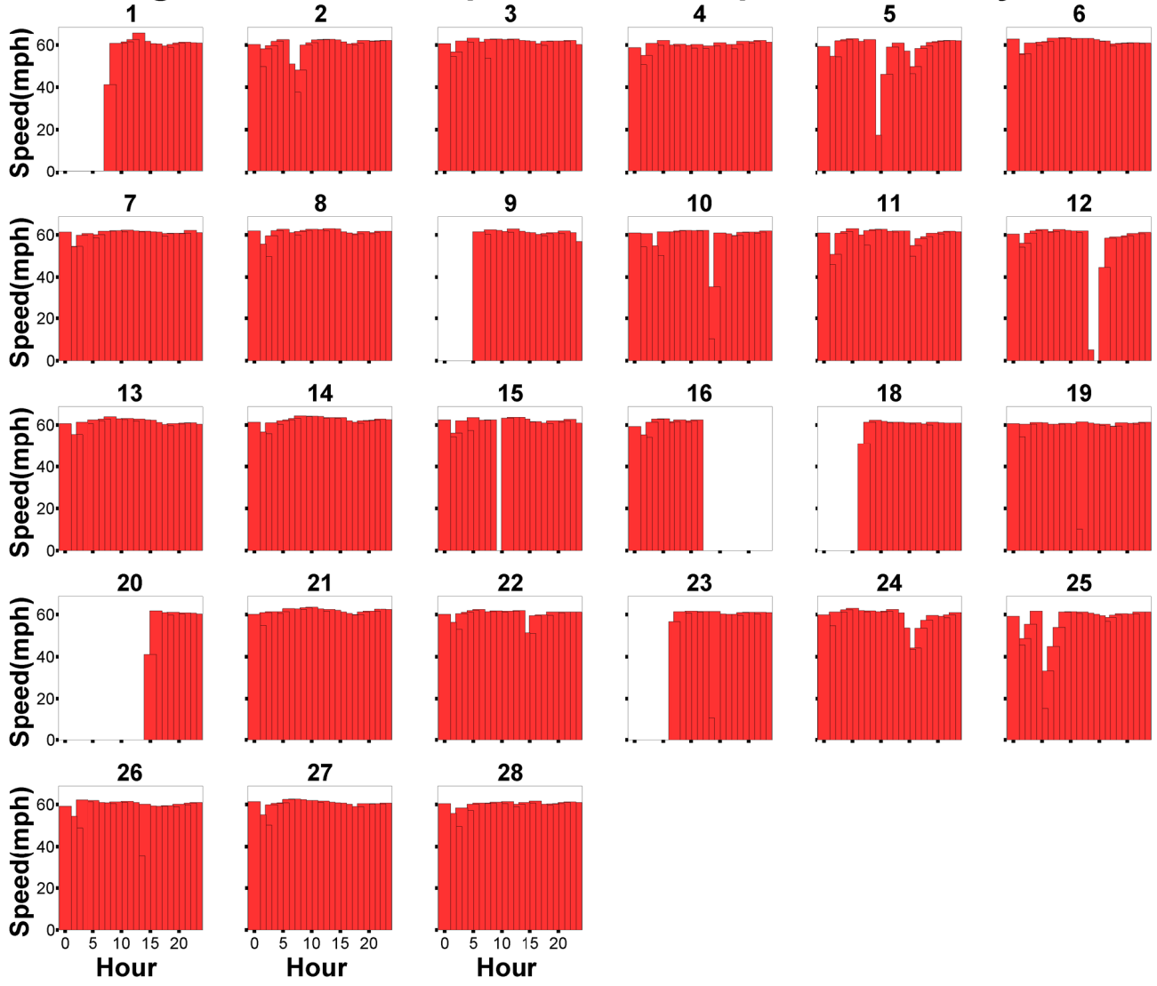
A4 Figure 3. Test Ramp: Detector A Speeds February 1999.
