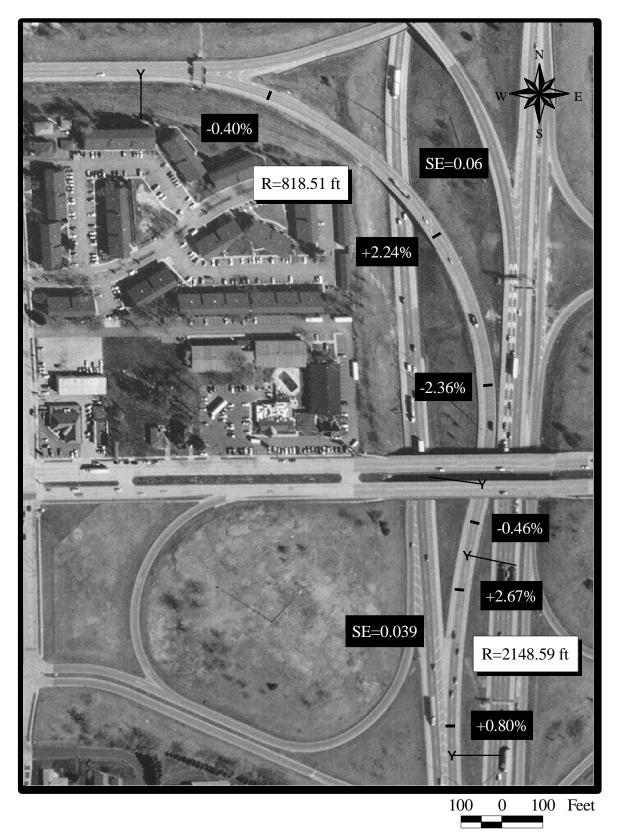
A3 Figure 4. Control Ramp Geometry.
