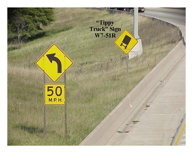
Figure 4. Warning Signs Near Test Ramp Point of Curvature.
