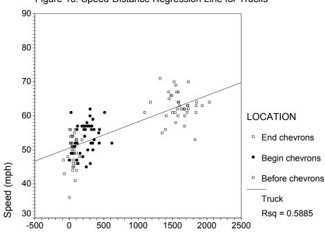
Figure 16. Speed-Distance Regression Line for Trucks
