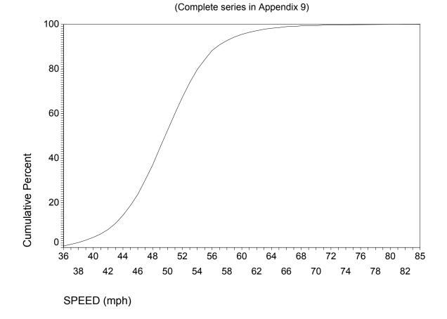
Figure 11. Detector B Cumulative Speed Distribution After Period
