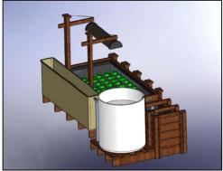
**Figure 4**. A cross-sectional view of the sump pump and plant tanks (left). A 3-D view from the rear showing the fish tank (cylinder) and the long rectangular tank for solids removal and biofilter (right).
