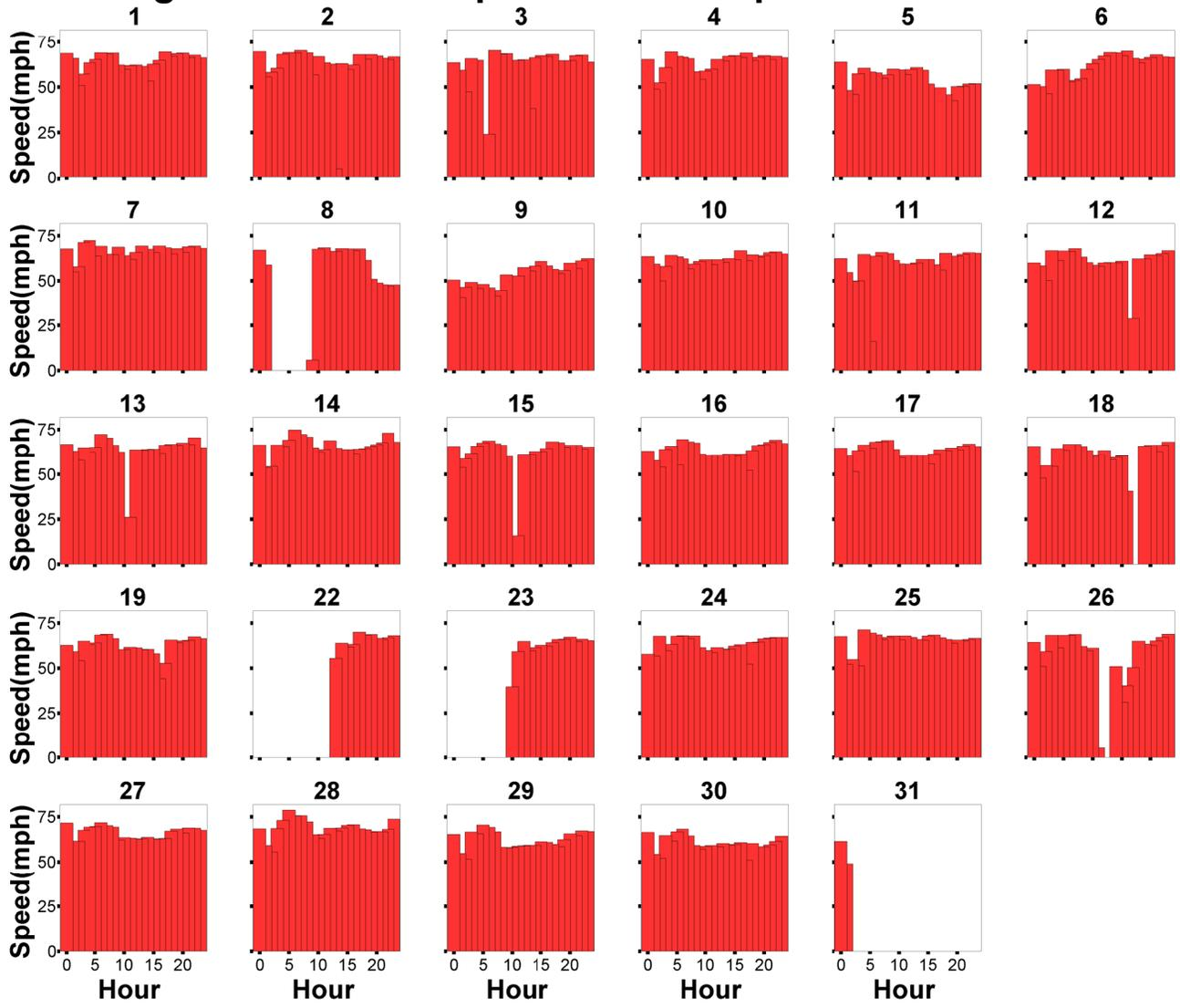
**A4 Figure 9. Control Ramp: Detector C Speeds December 1998.**
