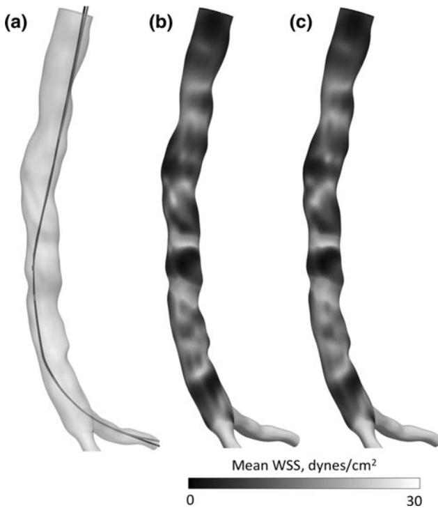
**FIGURE 13.** (a) Solid model with wire pathways reconstructed from 13 (black) and 41 (gray) candidate points per orthogonal plane. Distributions of mean WSS are nearly identical for vessels reconstructed with segments registered on pathways using 13 (b) as compared to 41 (c) candidate points.
