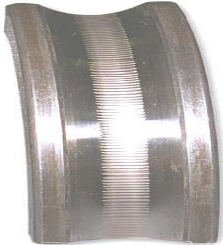
**Figure 1-4.** Bearing raceway with the signs of fluting, [15].
