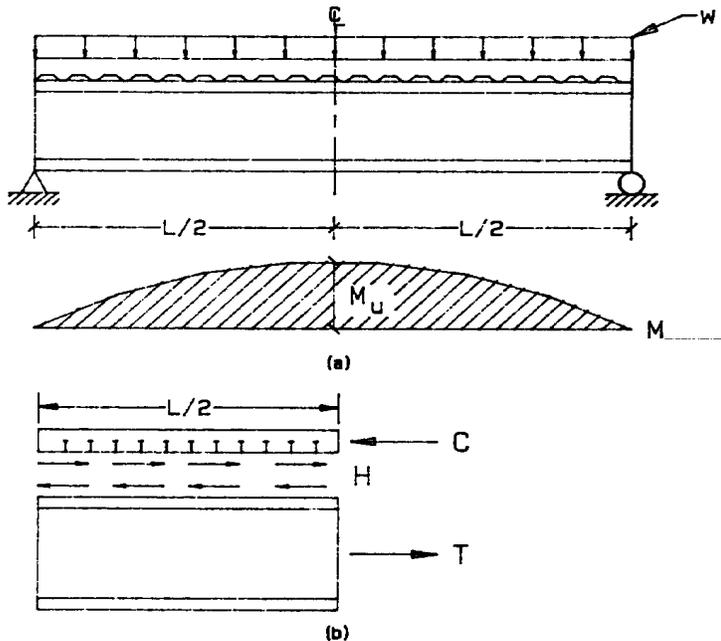
Fig. 3. Shear forces at ultimate moment
