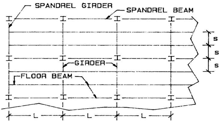
(a) Typical Floor Plan
