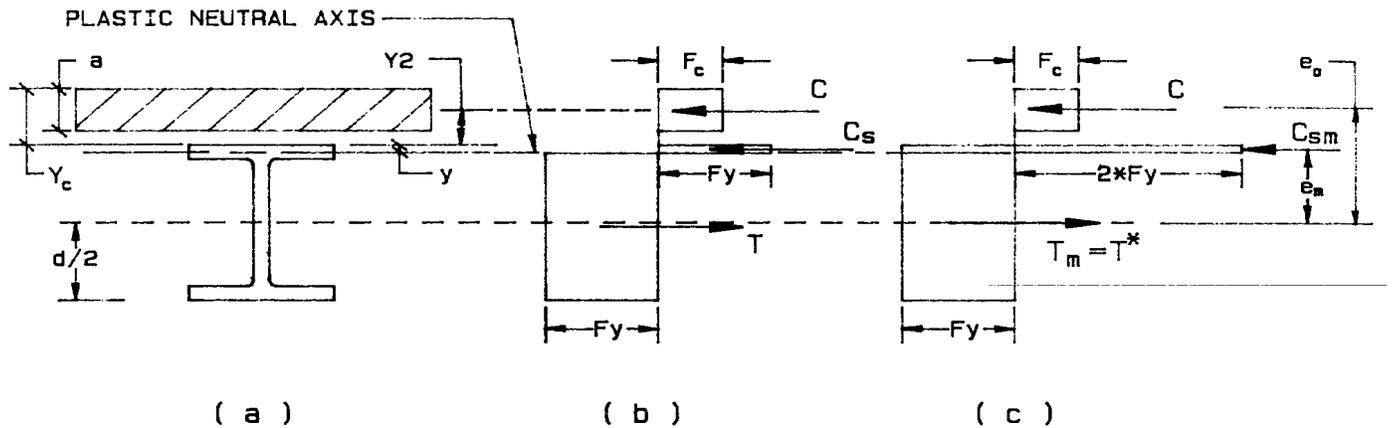
Fig. 5. Plastic neutral axis in flange (Case b)
