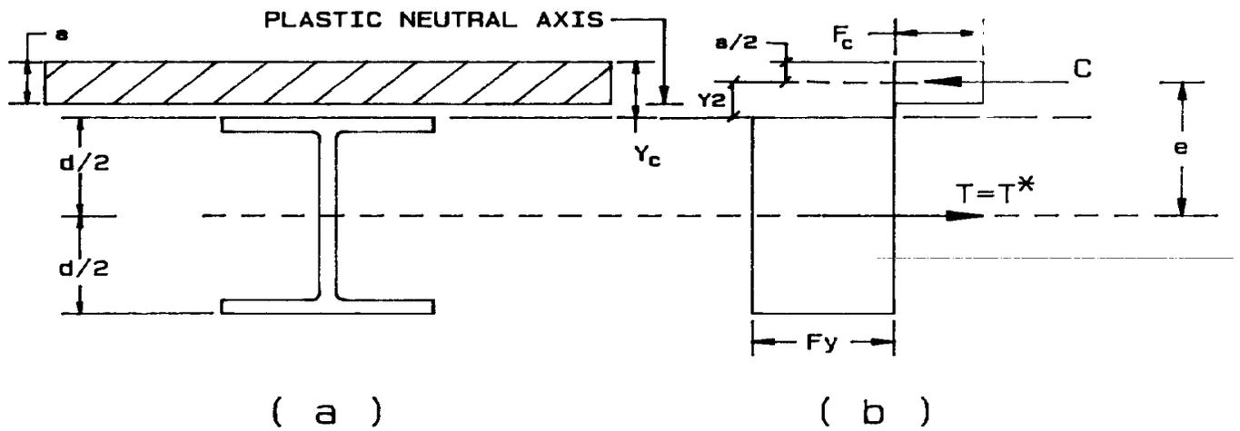
Fig. 4. Plastic neutral axis in slab (Case a)
