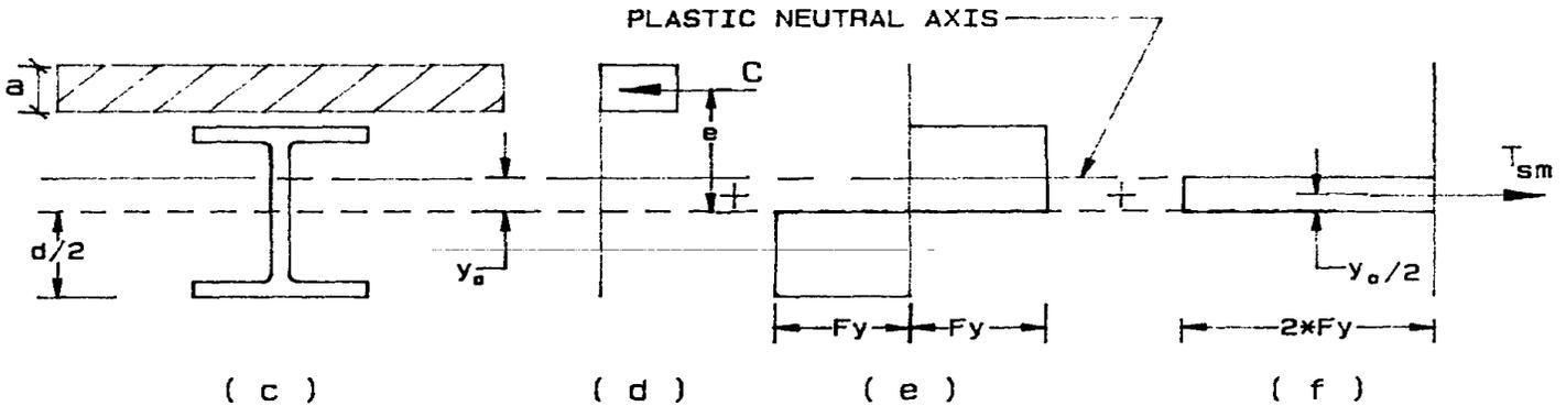
Fig. 6. Plastic neutral axis in web (Case c)
