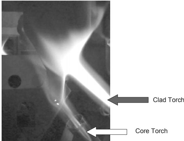
**Fig. 6: Typical Core and Clad Deposition in VAD Process.**
