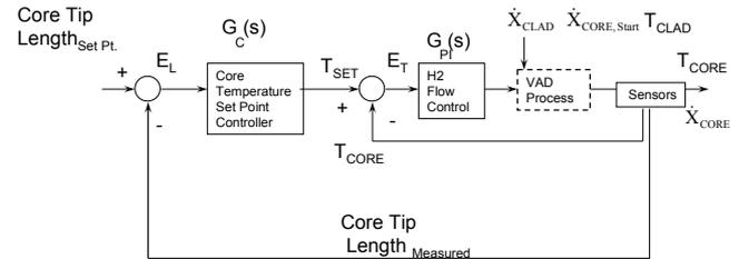
**Fig. 5: Proposed VAD cascaded control scheme, with an inner temperature control loop and an outer control for core tip soot, to provide a more uniform final product.**
