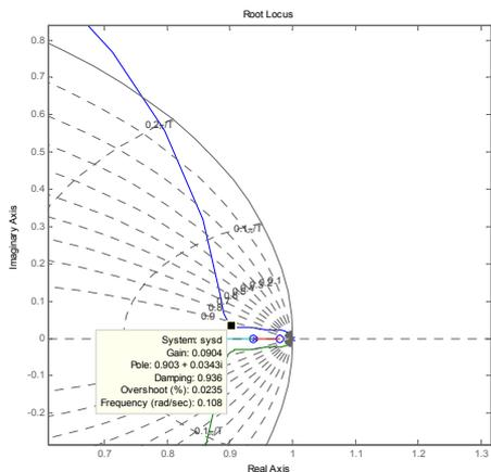
**Fig. 12: Discrete domain root locus for the core tip length transfer function with PI controller. Controller pole ( $K_i/K_p$ ) value is 0.02.**
