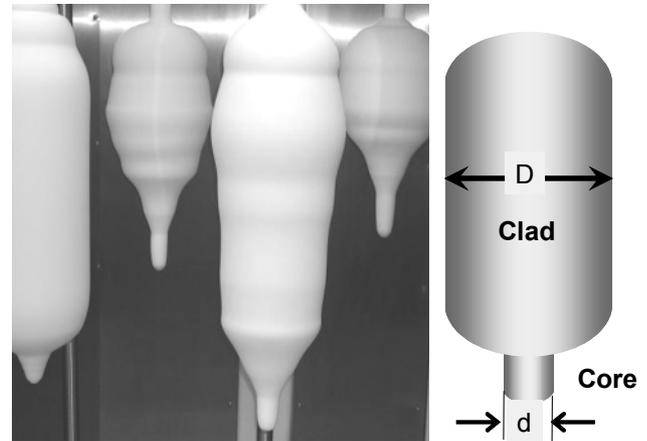
**Fig. 2: Variation in soot outside diameters and core tip length. (Core tip diameters depicted are nominally 40-mm.)**
