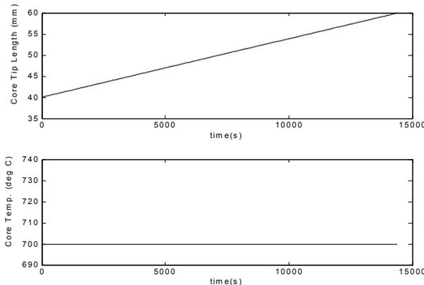
**Fig. 9: Open-Loop response of VAD process: Core tip temperature (top); core tip substrate temperature (bottom). Mismatched axial deposition rates for the core and clad torches are 65 and 60mm/hr, respectively.**
