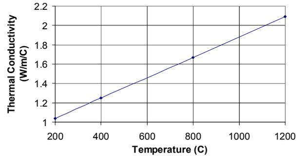
**Fig.7: Thermal conductivity of ceramic  $\text{SiO}_2$  [10].**
