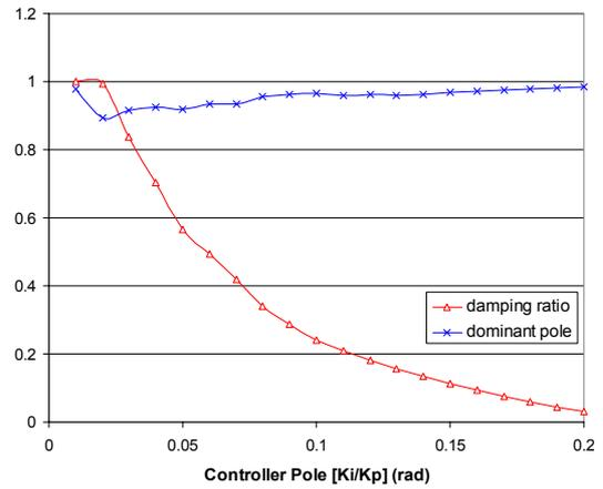
**Fig. 13: Damping ratio and dominant system pole for the closed-loop core tip length transfer function with PI controller vs. controller pole ( $K_i/K_p$ )**
