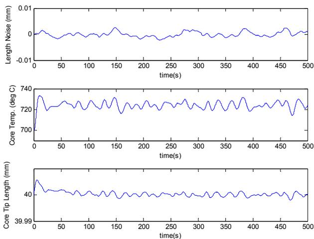
**Fig. 16: Simulation of closed loop system with sensor noise: sensor noise (top), temperature (middle), core tip length (bottom). Closed-loop response with PI-control of the core temperature control in the cascaded control scheme**
