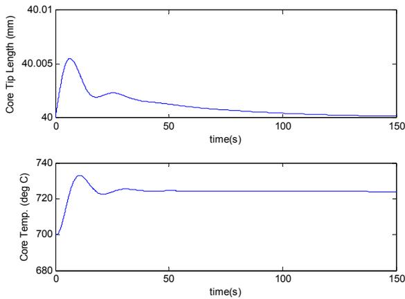
**Fig. 15: Closed-loop response of VAD process: core tip temperature (top); core tip substrate temperature (bottom) a proportional control gain magnitude of 6630°C/mm and an integral gain ratio of 0.020.**
