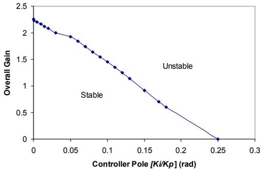
**Fig. 11: Stability limits for discrete domain root loci for the open-loop core tip length transfer function with PI controller.**
