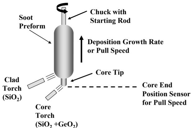
**Fig. 1: VAD process depicting core and clad torches depositing glass soot onto the rotating preform. The core tip position is held constant causing the preform and chuck to move upward.**
