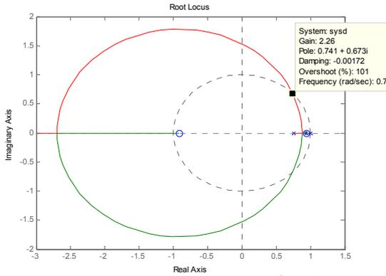
**Fig. 10: Discrete domain root locus for the open-loop core tip length transfer function with the embedded temperature control.**
