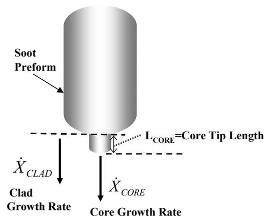
**Fig. 3: Core and clad growth rates for soot preform creation.**
