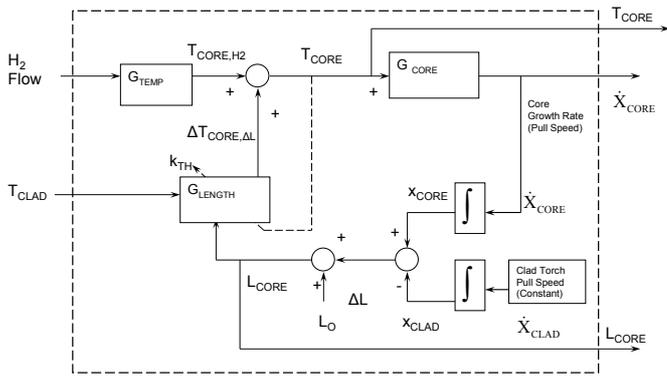
**Fig. 8: System model block diagram of the core soot substrate temperature and growth.**
