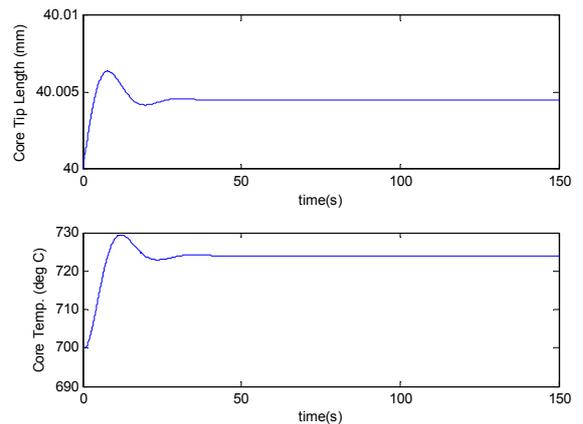
**Fig. 14: Closed-loop response of VAD process: core tip temperature (top); core tip substrate temperature (bottom) with a proportional control gain magnitude of 5355°C/mm (overall system gain of 0.073).**
