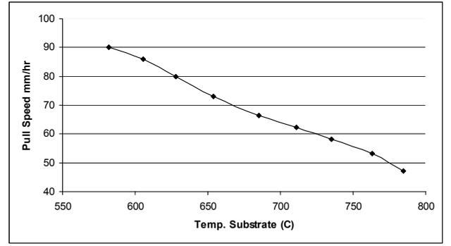
**Fig. 4: Experimental data for pull speed (core growth rate) vs. soot perform core tip substrate temperature. An approximately linear relationship exists between pull speed and core tip temperature.**
