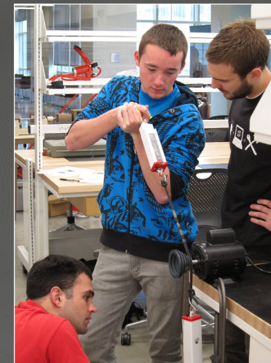
Measuring Belt Tension
