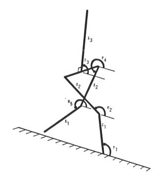
Figure 1. Bipedal Locomotion Model.
