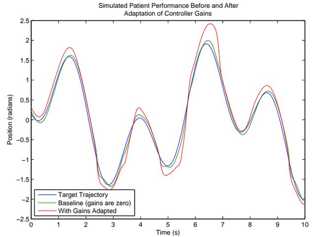
**FIGURE 9. SIMULATED HEALTHY PATIENT PERFORMANCE BEFORE AND AFTER CONTROLLER GAINS ARE ADAPTED**
