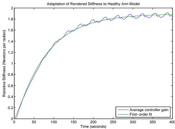
**FIGURE 8. RENDERED STIFFNESS BEING ADAPTED TO HEALTHY PATIENT PERFORMANCE (SIMULATED)**
