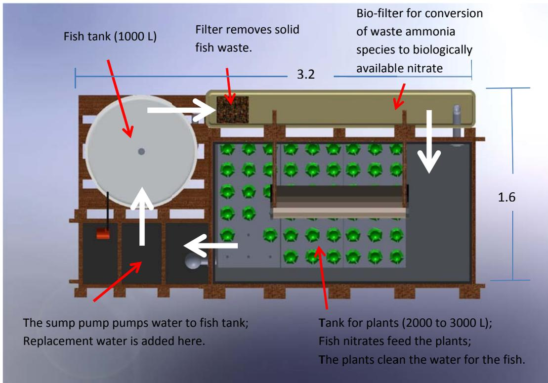
**Figure 2.** Top view of a small aquaponics system with descriptions of components. The white arrows represent the flow of water.
