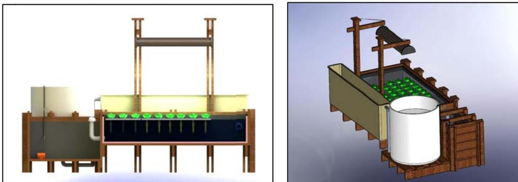
**Figure 4.** A cross-sectional view of the sump pump and plant tanks (left). A 3-D view from the rear showing the fish tank (cylinder) and the long rectangular tank for solids removal and bio-filter (right).
