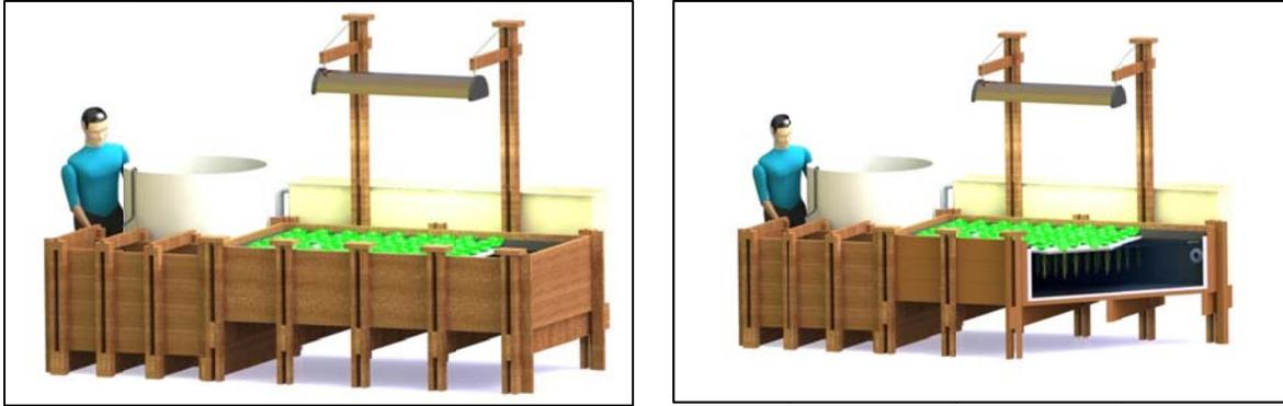
**Figure 3.** A 3-D drawing of the small aquaponics system (left). A cut-away view of the water tank for plants (right).
