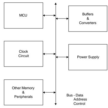
•Buffers: condition I/O to proper levels •Bus: data, address, control signals •Clock: Fixed-frequency timing signal •MCU: CPU, Memory, Registers connected by internal bus -CPU: controls microcontroller operations -Memory: program & data storage •ROM, RAM, EEPROM -Registers: temporary storage for data manipulation
